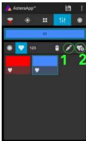
To add a color to the favorites, press (2). To edit an existing favorite color, select it and press the pen (1).
